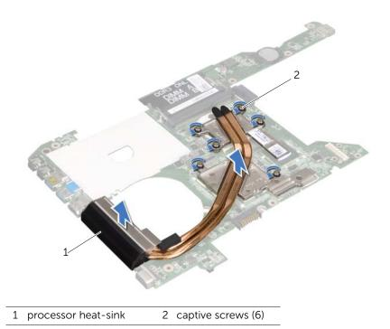
Replacing the Processor Heat-Sink
