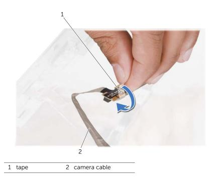
4 Disconnect the camera cable from the connector on the camera module.
