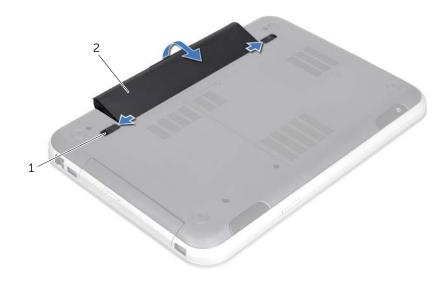
1 battery release latches (2) 2 battery
