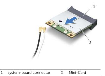
CAUTION: When the Mini-Card is not in the computer, store it in protective antistatic packaging. For more information, see "Protecting Against Electrostatic Discharge" in the safety information that shipped with your computer.
